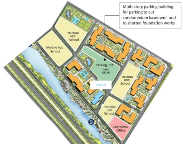
Figure 14: Typical mid-range Vinhomes condo section layout – parking unit to cut basements out of condominium buildings
